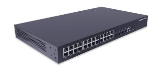
providing flexible connectivity options. With a PoE power budget of up to 400W, it can reliably power connected devices. The switch has a switching capacity of 128Gbps, ensuring efficient data transmission and high-performance networking.
